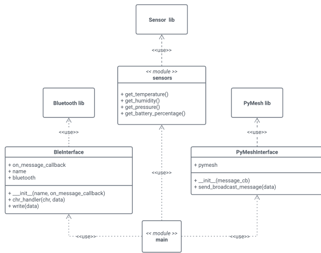
Fig. 2. Class diagram of the micropython code executed in the fipy
