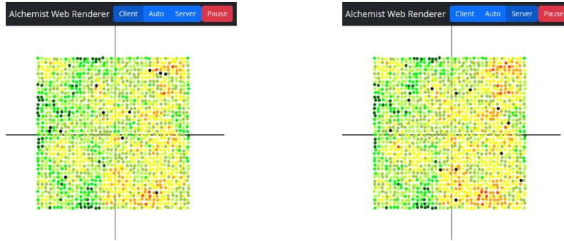
Fig. 6: Snapshots of the monitor/controller UI for the proof-of-concept, taken subsequently during the same experiment. Initially (left) the render (i.e., \mathcal{H} ) is running within the client’s browser (i.e., \mathcal{N} ), then (right), at runtime, it is migrated to the server (i.e., \mathcal{F} ), with no interruption, and no perceivable difference in the rendered image. In both snapshots, the warmer the color, the more the corresponding node had resource availability for itself.
