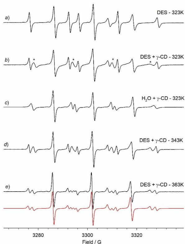
Figure 1. EPR spectra of BTBN recorded in DES at 323K (a) and in the same solvent in the presence of \gamma -CD 50 mM at 323K (b), 343 K (d), 363 K (e). Spectrum (c) was obtained in water at 323 K in the presence of 50 mM \gamma -CD. As an example, in red is reported the theoretical simulation of spectrum (e) obtained by using k_{on} = 8.8 \times 10^7 \text{ s}^{-1} \text{ M}^{-1} , k_{off} = 3.8 \times 10^6 \text{ s}^{-1} . Asterisks in spectrum (b) correspond to clean EPR lines deriving from the included radical.
