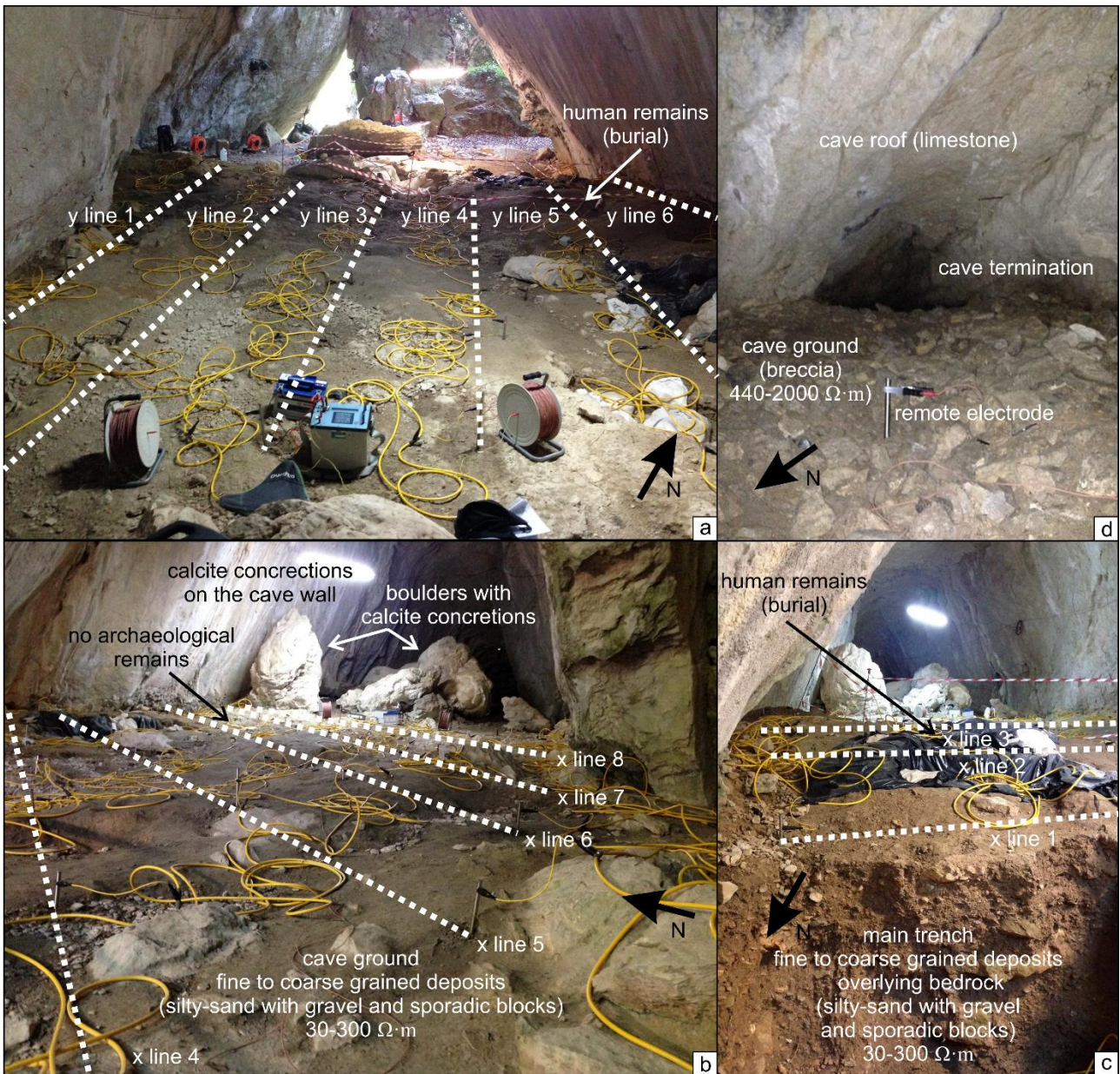
1089 Fig. 4: Pictures showing different views of the 3D ERT survey grid along with lithological
