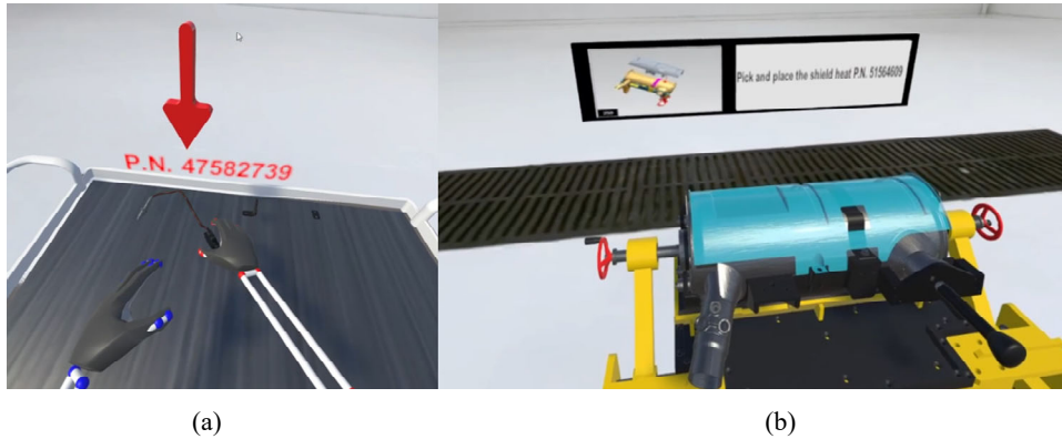
Figure 1 Examples of KTFs, (a) arrow guideline and part number (b) SOP instruction and ghost guideline (see online version for colours)
