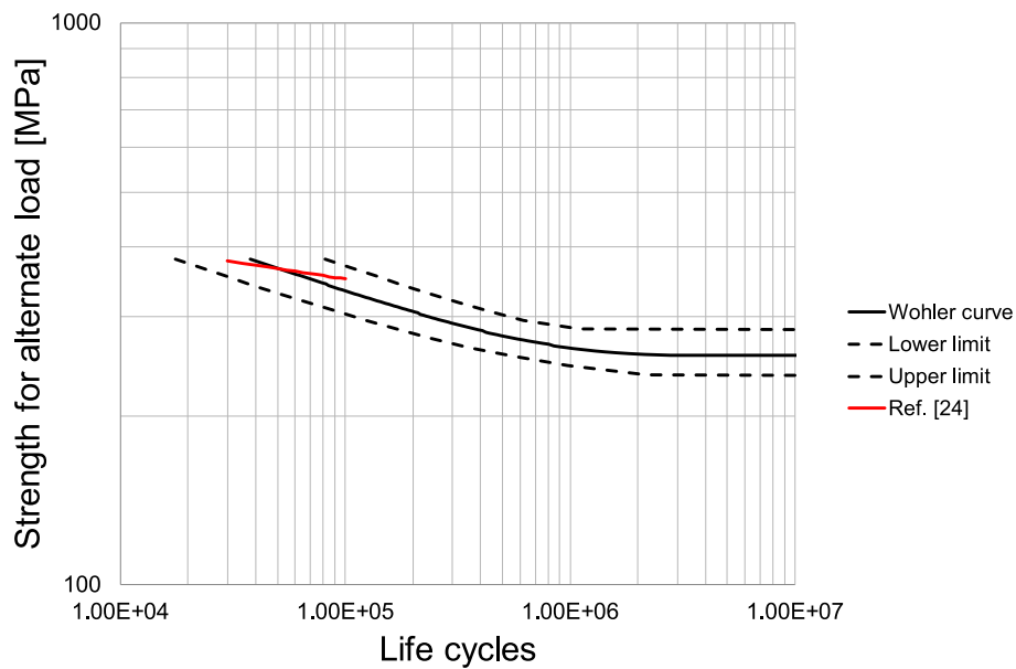
Fig. 7. Wöhler curve: strength for alternate symmetric load plotted vs. lifespan for EUROFER97 following the novel treatment and the conventional one [24].
