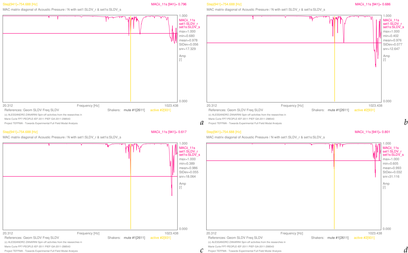
Figure 26. MACii graphs in the comparison of the acoustic transfer matrix as in Equations (14) and (18), at specific distances of 25 mm in (a), 75 mm in (b), 150 mm in (c), and 300 mm in (d) at the specific frequency of 755 Hz, with excitation from shaker 2.
