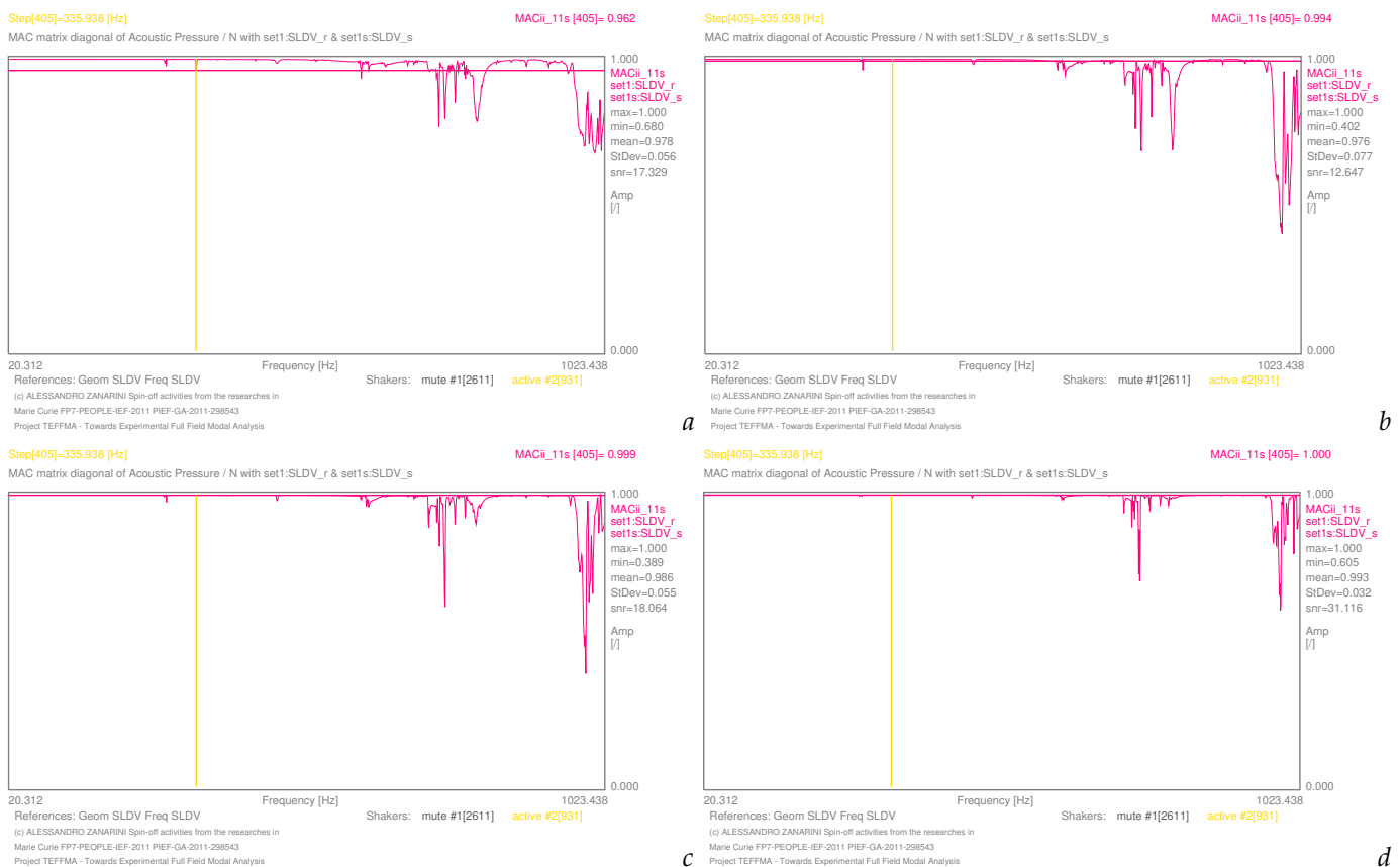
Figure 21. MACii graphs in the comparison of the acoustic transfer matrix as in Equations (14) and (18), at specific distances of 25 mm in (a), 75 mm in (b), 150 mm in (c), and 300 mm in (d) at the specific frequency of 336 Hz, with excitation from shaker 2.
