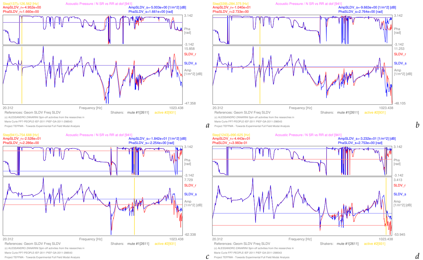
Figure 3. Vibro-acoustic FRFs in acoustic dof 941, obtained in Equations (14) and (18) from raw (red) and smoothed (blue) receptances respectively, in the [20–1024] Hz frequency range at specific distances of 25 mm (a), of 75 mm (b), of 150 mm (c) and of 300 mm (d) from shaker 2 in structural dof 931.
