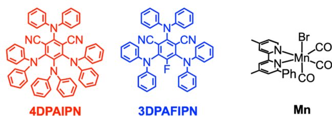
Chart 1. Structures of the molecules exhibiting thermally activated delayed fluorescence (4DPAIPN and 3DPAFIPN) and catalyst (Mn) used in this study.
