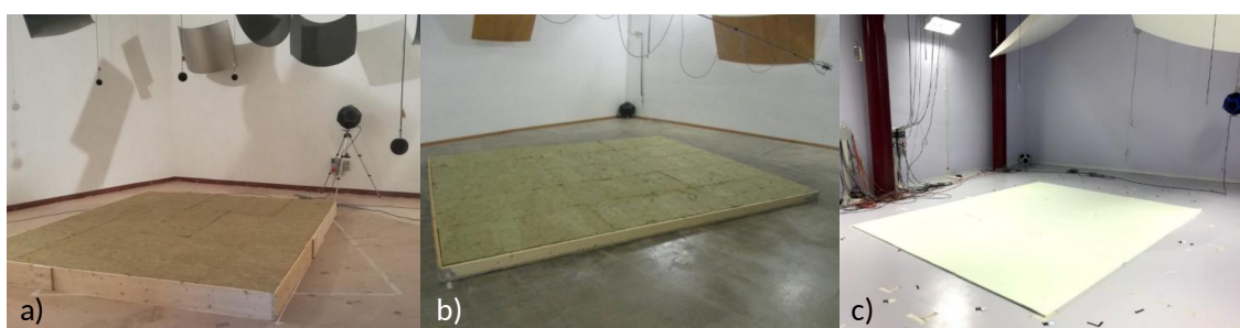
Figure 3 - Photographs of the three samples under test in three different laboratories participating in the ILT: a) 20 cm sample; b) 10 cm sample; c) 2 cm sample
