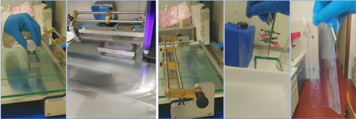
Supplementary Figure 4. Manufacturing process to obtain thin sheets of siloxane scintillator, photographed in its main steps. From left to right: pouring of the resin with additives into the film applicator (500 \mu\text{m} gap), casting with motorized stage, immersion in water of the vulcanized material and stripping from the glass plate, ultimately leading to dried, self-supporting foil of siloxane scintillator ready to be cut to size.
