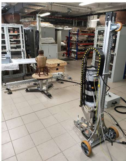
Fig.3: (left) the CT system installed in the basement of the Museum; (right) a schematic of the system.
