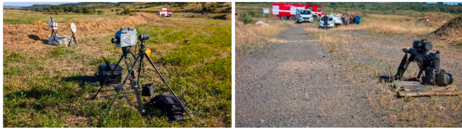
Fig. 2. Experimental equipment set-up, high-speed and infrared cameras (left), shooting position (right).
