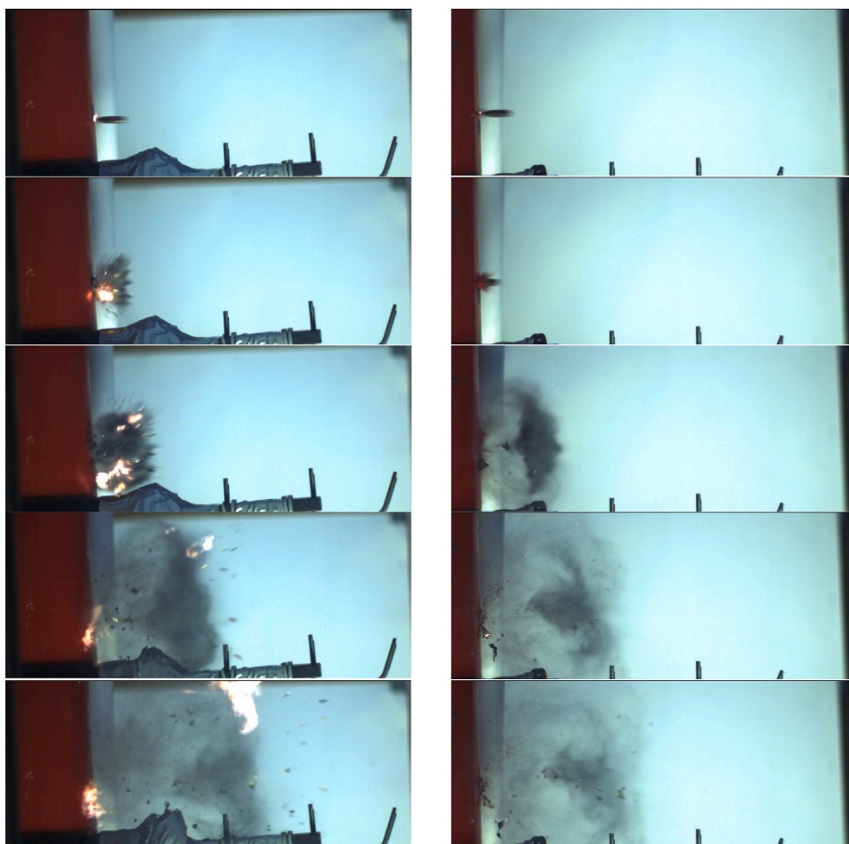
Fig. 6. Hydrogen release with ignition (left) and non-ignition (right).
