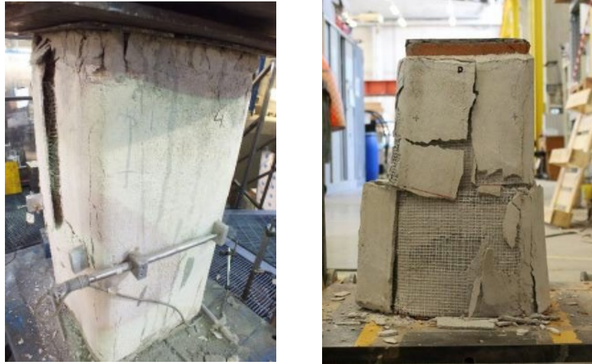
619 Fig. 22. Failure mode of clay brick masonry specimens confined by SRG.
