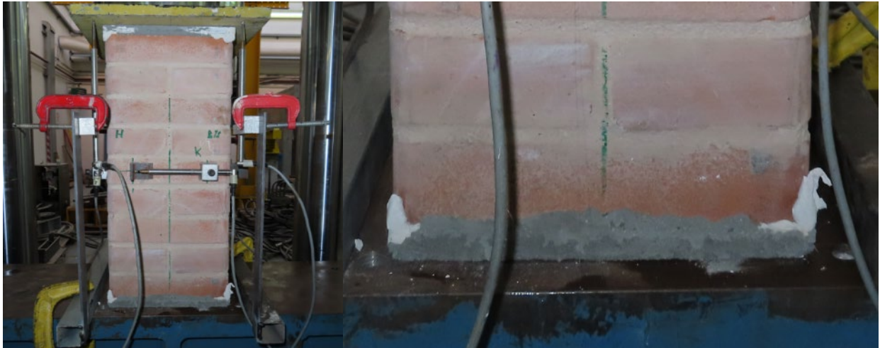
270 271 Fig. 6. Mortar layers placed on top and bottom face of masonry specimens (UniNa).
