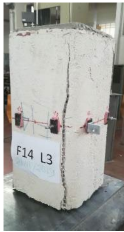
418 Fig. 11. Failure mode of Tuff masonry specimens confined by GFRCM.
