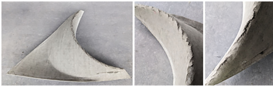
Fig. 6 Preliminary folding tests of fiber cement boards displayed fractures and crimps in the areas around the sharp creases
