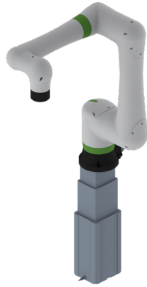
Fig. 4. Cobot mounted on a telescopic column.
