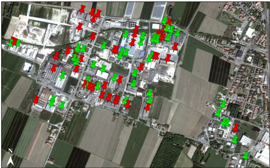
Fig. 5 Google Earth (2021) aerial view with the position of the precast buildings. In red the buildings collapsed during the 29th May 2012 main shock
