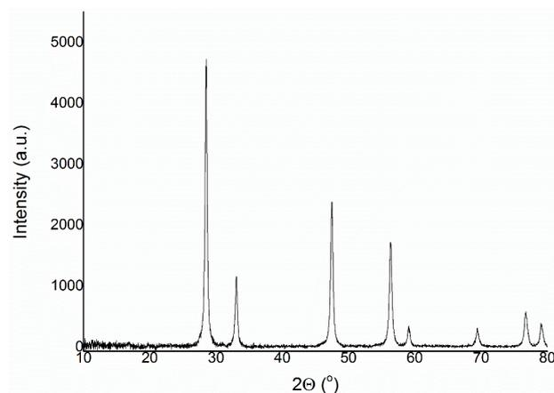
**Figure 2.** X-Ray diffraction pattern for Ir/CeO<sub>2</sub>
