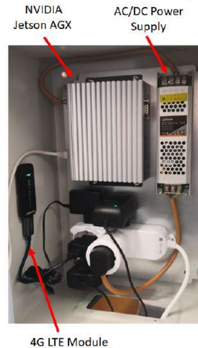
Fig. 6: Prototype of the mobility monitoring sub-system.
