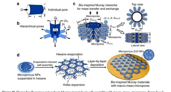
**Figure 49.** Hierarchically porous networks in Murray materials via self-assembly with macro–meso–micropores. Reproduced from [470]. CC BY 4.0.
