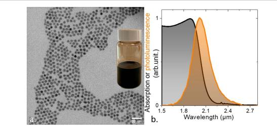
**Figure 11.** (a) Transmission electron microscopy image of infrared nanocrystals. The inset is an image of a vial containing a colloidal solution of infrared absorbing nanocrystals. (b) Absorption and photoluminescence spectra of short-wave infrared active HgTe nanocrystals.
