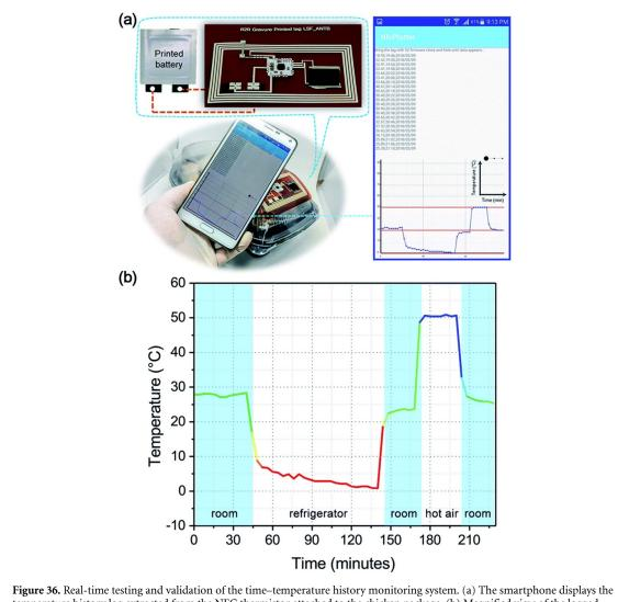
temperature history monitoring system. (a) The smartphone displays the temperature history monitoring system. (a) The smartphone displays the temperature history log extracted from the NFC thermistor attached to the chicken package. (b) Magnified view of the logged temperature data under different conditions. Reproduced from Ref. [366] with permission from the Royal Society of Chemistry.
