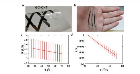
**Figure 39.** Graphene oxide-CNT temperature sensor. Photos of sensors (a) under bending and (b) on a hand. (c) Resistance and (d) normalized resistance as a function of temperature. Reprinted with permission from [391]. Copyright 2021, American Chemical Society.
