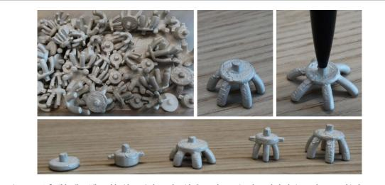
Figure 65. A flexible silver/silver chloride EEG electrode with *fingers* for passing through the hair. Work reported in [617, 618].
