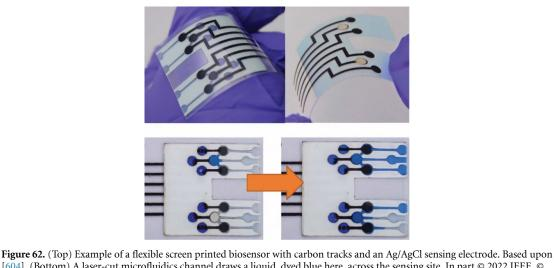
[604]. (Bottom) A laser-cut microfluidics channel draws a liquid, dyed blue here, across the sensing site. In part © 2022 IEEE. © 2022 IEEE. Reprinted, with permission, from [604].
