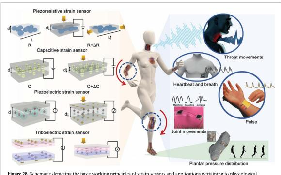
Figure 28. Schematic depicting the basic working principles of strain sensors and applications pertaining to physiological bio-signals in the body. Reprinted from [287], Copyright 2022, with permission from Elsevier.
