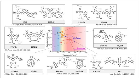
Figure 6. Detectivity, or signal-to-noise ratio, of organic near-infrared/SWIR detectors, along with the corresponding molecular structures.
