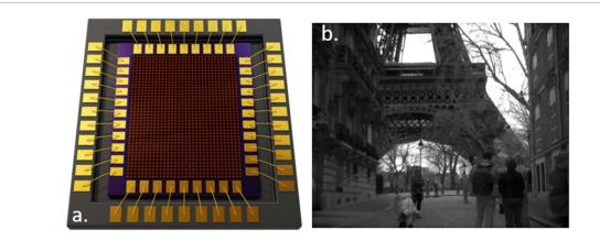
**Figure 12.** (a) Schematic of a ROIC functionalized by a nanocrystal film to sensitize it in the infrared. (b) Image of the Eiffel tower taken with a HgTe nanocrystal-based infrared camera with 2  $\mu$ m cut-off wavelength. Adapted with permission from [115]. Copyright 2023 American Chemical Society.
