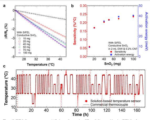
**Figure 40.** CNT-SnO<sub>2</sub> temperature sensor. (a) Resistance change ratio at different  $SnO_2$  compositions in a CNT ink and at different temperatures. (b) Sensitivity and activation energy of the sensor with different  $SnO_2$  compositions. (c) Long-term temperature monitoring compared to the output of a commercial thermocouple used in a temperature-controllable oven. Reproduced with permission. [390] Copyright 2019, John Wiley & Sons.
