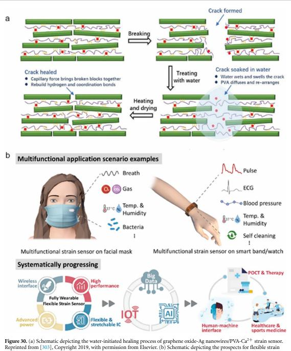
**Figure 30.** (a) Schematic depicting the water-initiated healing process of graphene oxide-Ag nanowires/PVA-Ca<sup>2+</sup> strain sensor. Reprinted from [303], Copyright 2019, with permission from Elsevier. (b) Schematic depicting the prospects for flexible strain sensors in regards of physiological signal monitoring and integration of multiple systems. Reprinted from [287], Copyright 2022, with permission from Elsevier.
