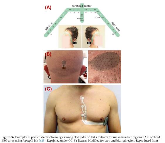
EG array using Ag/AgCl ink [625]. Reprinted under CC-BY license. Modified for crop and blurred region. Reproduced from [625]. CC BY 4.0. (B) Temporary tattoo electrode for EEG, inkjet printed using PEDOT:PSS based ink on a polyurethane substrate. Reprinted under CC-BY license. Modified for crop. Reproduced from [612]. CC BY 4.0. (C) Chest ECG array using Ag/AgCl ink on a polyurethane substrate. © 2016, IEEE. Reprinted, with permission from [624].
