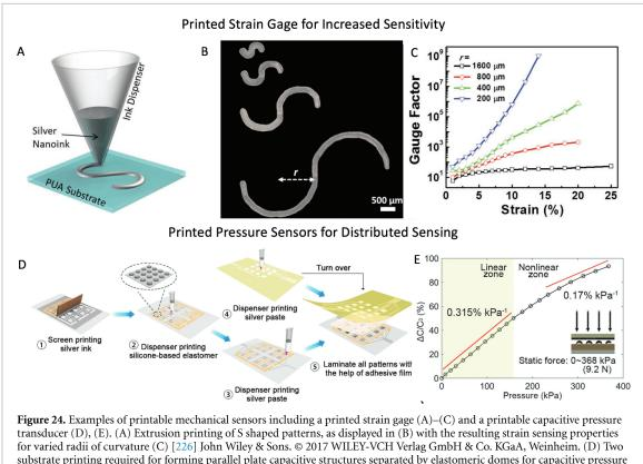
substrate printing required for forming parallel plate capacitive structures separated by elastomeric domes for capacitive pressure sensing, including the results displayed in (E). [227] John Wiley & Sons. © 2021 Wiley-VCH GmbH.
