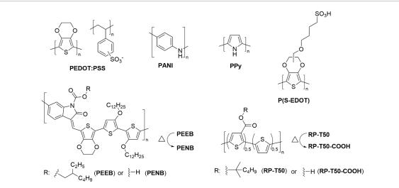
**Figure 35.** Representative conjugated polymers used for temperature sensors reported in the literature: poly(2,3-dihydrothieno-1,4-dioxin)-poly(styrenesulfonate) (PEDOT:PSS) [358], polyaniline (PANI) [359], polypyrrole (PPy) [359], P(S-EDOT) [360], PEEB/PENB [361], and RP-T50/RP-T50-COOH [362].
