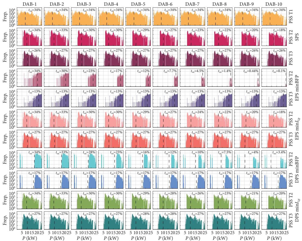
Figure 12 Histogram of the power allocation strategies of even sharing, efficiency-oriented module shedding, and module shedding with rotation per event under SPS, EPS, and DPS with minimum BFP and peak current schemes. Dashed lines indicate the position of average power and t_{on} is the active time in percentage.
