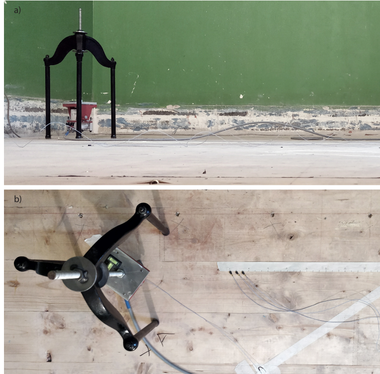
Figure 3: Experimental setup used to investigate the CLT floor installed in the laboratory facility. a) side view: the shaker is mounted on a tripod with rubber supports on the three feet; b) top view: three accelerometers are mounted along a wave propagation direction in line with the excitation point.
