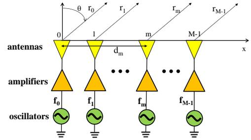
Fig. 1. Scheme of a standard FDA arrangement.
