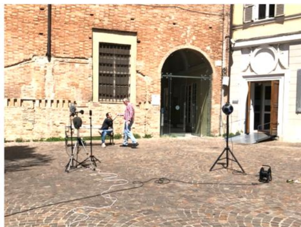
Fig. 6 Acoustic equipment deployed in Piazzale San Francesco for the acoustic survey
