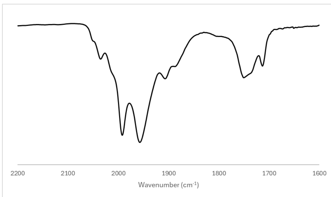
Figure S3. IR spectrum in the \nu_{\text{CO}} region of [\text{NEt}_4]_3[\text{HRu}_8(\text{CO})_{24}\text{Cu}_6\text{Br}_2] ( 4 ) in \text{CH}_2\text{Cl}_2 .
