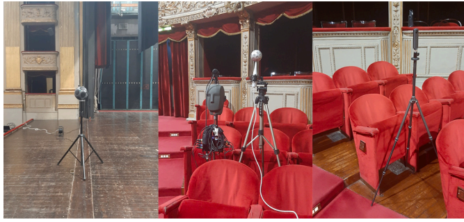
Fig. 2. Equipment setup: sound source (Look Line 103); receiving microphone combination; 360° camera (Ricoh Theta V).
