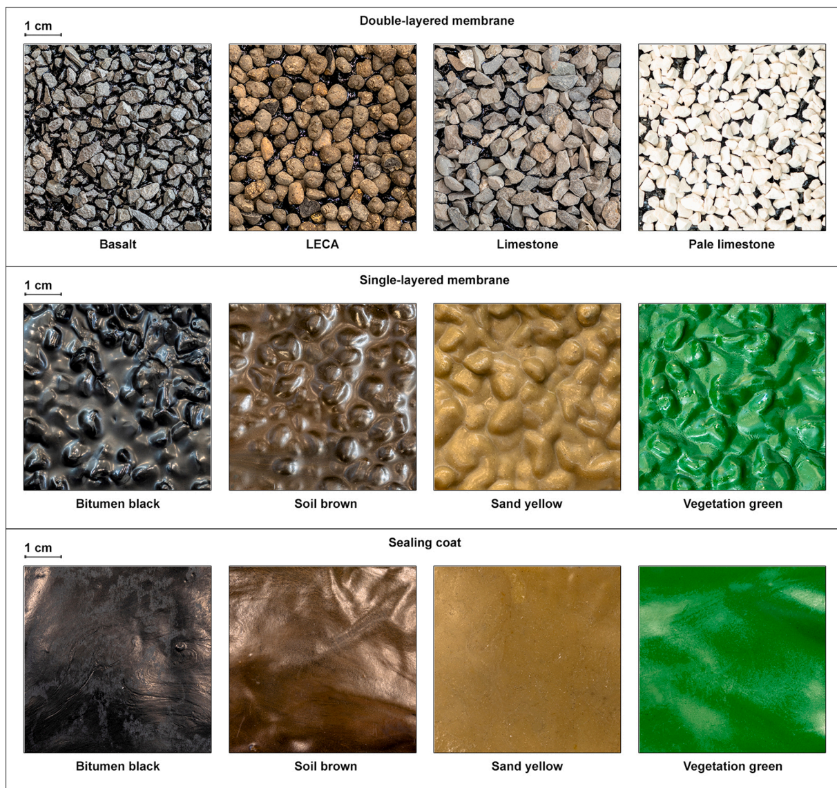
Fig. 9. Surface appearance of sealing treatments: (top) double-layered membranes with different finishing aggregates; (centre) single-layered membranes with different finishing binder; (bottom) sealing coats.
