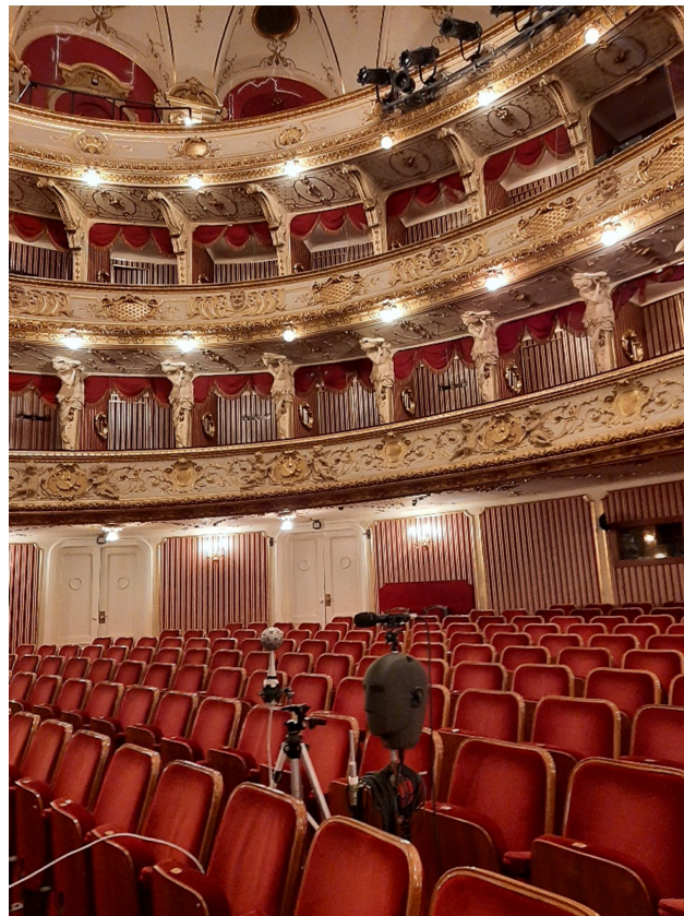
Figure 3. View of the equipment installed in the stalls during the acoustic measurements.
