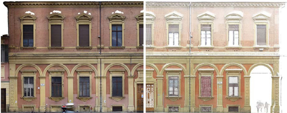
Figure 3. (On the left the mesh generated by the photogrammetric survey, on the right the point cloud from the laser scanner survey © Stefanini)
