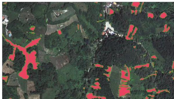
Fig. 2. Example of a dataset representing landslides manually segmented in the region of Broni (Italy).
