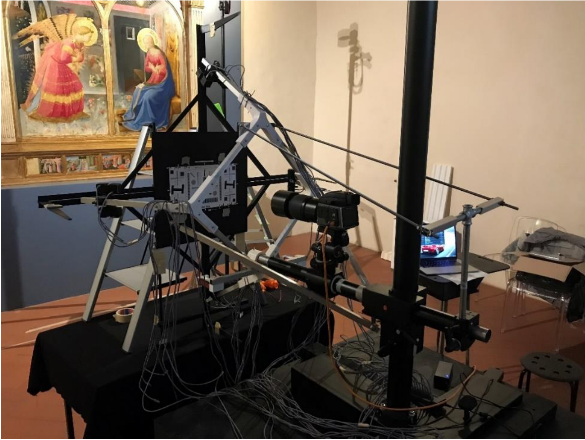
Figure 3. The custom stand mounting the light sources positioned at 45^\circ and 15^\circ relative to the painting's plane.
