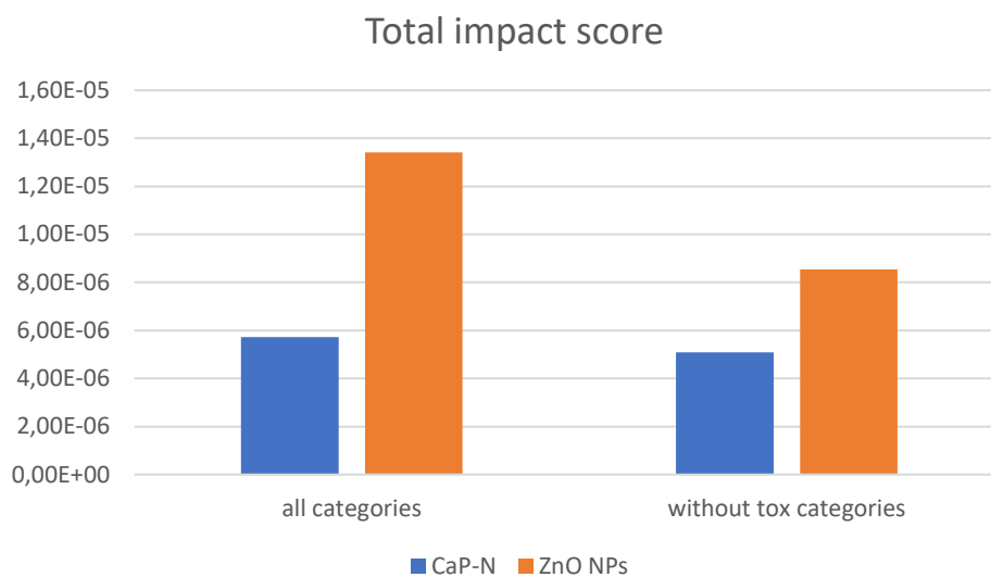
227 Figure 8. Comparison between the environmental impact of CaP-N and ZnO NPs production after 228 normalization and weighting.
