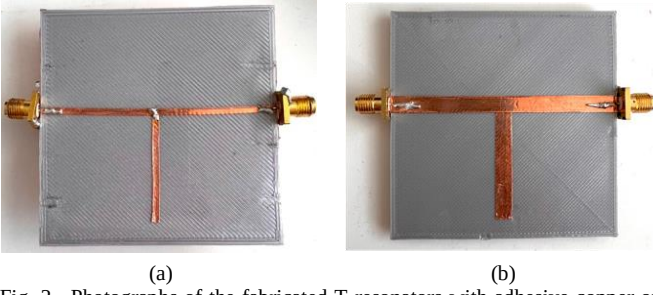
Fig. 2. Photographs of the fabricated T-resonators with adhesive copper on (a) 0.5 mm and (b) 2-mm-thick PLA samples.
