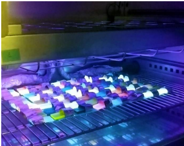
Fig. 3 Samples during the ageing inside the climate chamber
