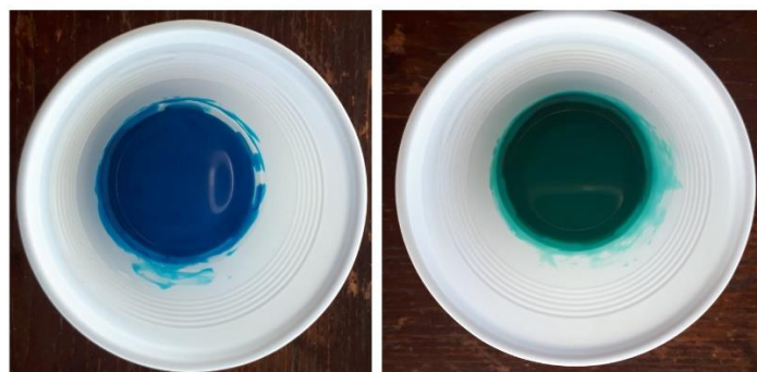
Fig. 2 Images show Epo-Tek 301-2 with blue Orasol before and after the hardener was added.
