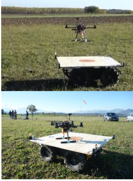
Fig. 1. Experimental tests of drone landing on mobile platforms.
