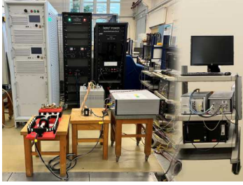
Fig. 1. PTB laboratory setups of the reference measurement system for CT and LPCT characterization in presence of PQ disturbances.
