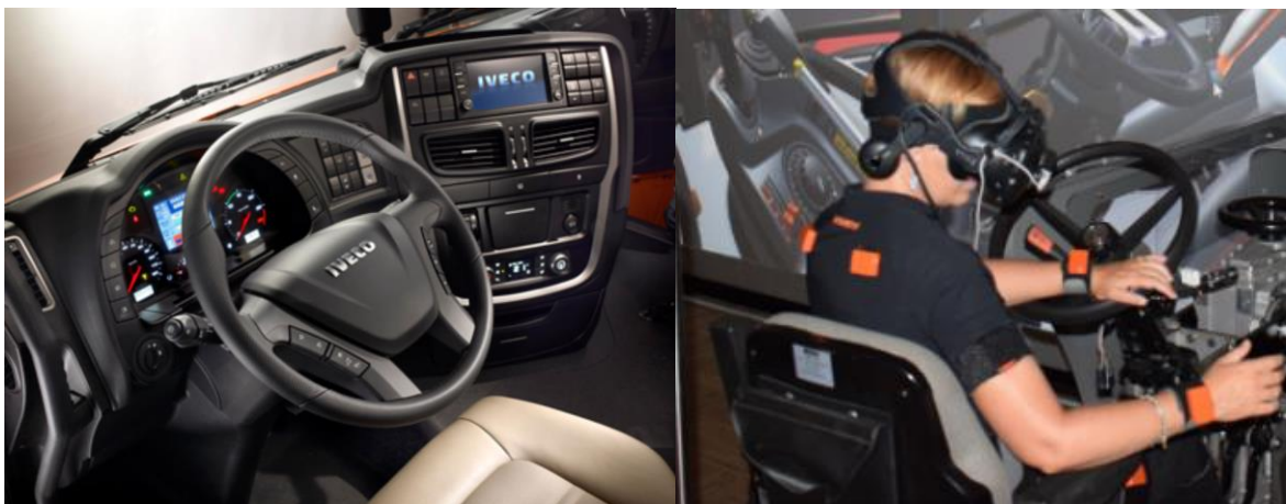
Fig. 9. UC2 Phase 3: new control layout based on intuitive-grouped control panel (left) and immersive VR test in Lab (right)
