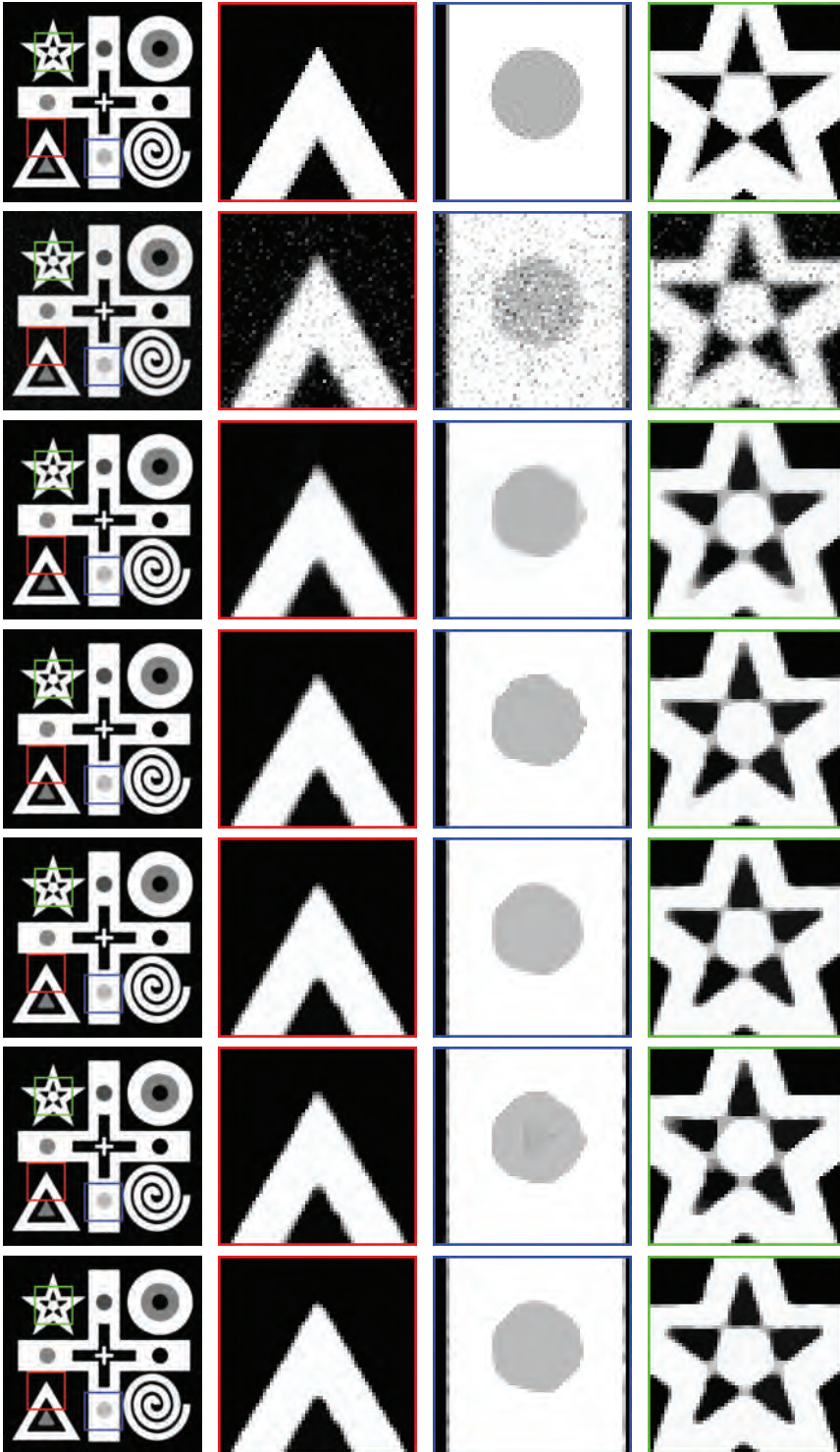
Fig. 19 From top to bottom: for the test image geometric , original image, observed image b , performance of the TV, the TV_p (with output p = 0.5 ), the WTV, the WTV_p^{sv} , and the WDTV_p^{sv} regularizers with the respective close-up(s).
