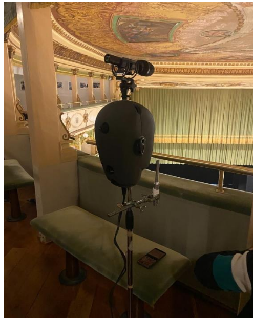
Figure 5. Complete set up including B-Format microphone, an omnidirectional microphone and a dummy head.
