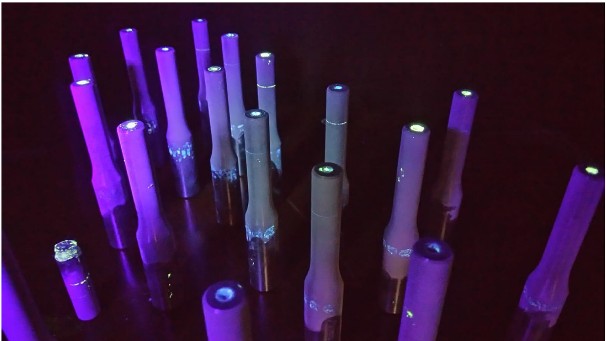
Figure 5 – Dye penetration inspection on the shaft specimens
