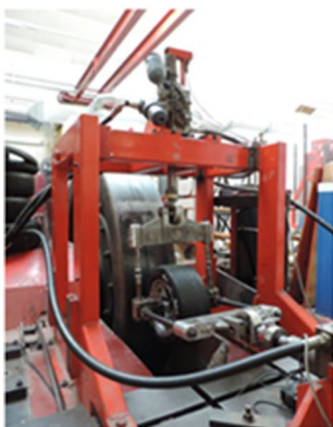
Fig. 23 Indoor tire test rig
