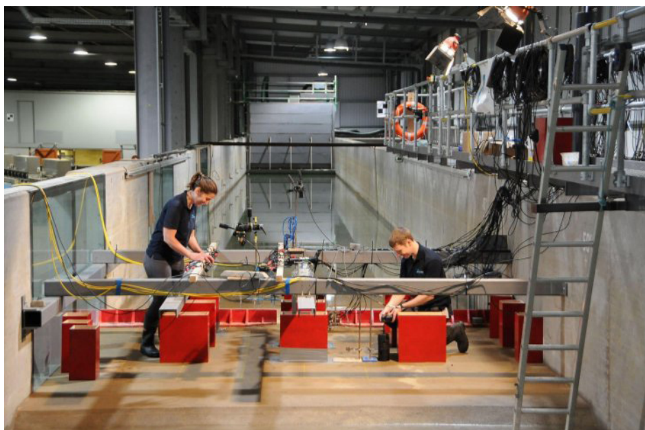
Figure 6. HR Wallingford's Froud Modelling Hall. The picture shows the 4m wide Fast Flow Facility during tests conducted for URBANWAVES, with the Tsunami Simulator seen at the far end of the flume.
