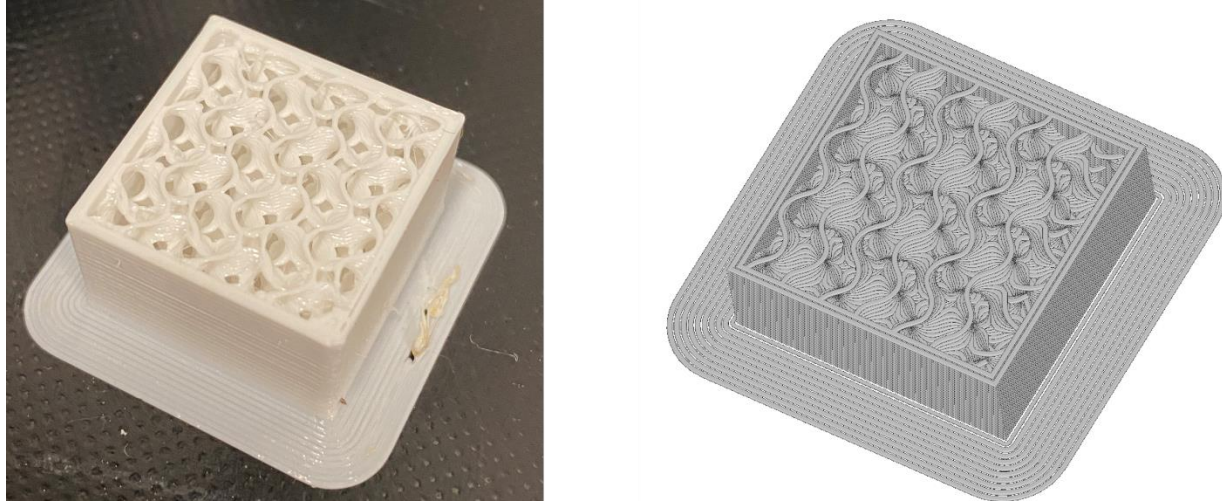
Fig. 9. Comparison of real geometry (left), and reconstructed geometry in FreeCAD (right).
