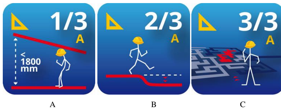
Fig. 1. Conditions of geometric confinement (A. Presence of at least one dimension of the space < 1800 mm; B. The space presents hollow areas, below the walking surface; C. The space is extended or branched in various areas, with hollow surfaces)
