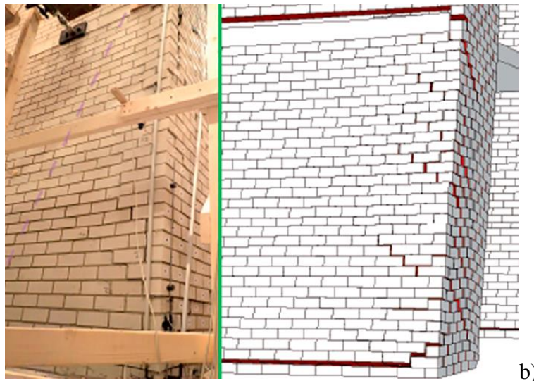
872 Figure 18 –Numerical examples of tothing behavior: (a) continuum micromodel considering the bricks 873 and mortar separately, and (b) damaging block-based model with cohesive-frictional contact (D’Altri et 874 al. 2019).
