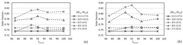
**Figure 3.** Solar fraction achieved with the proposed logic as a function of control settings. Data reported for  $T_{set, TES} = 90^{\circ}$ C (a) and  $T_{set, TES} = 95^{\circ}$ C (b).
