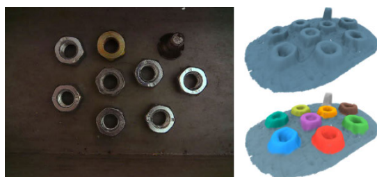
FIGURE 10. Reconstruction (top right) of a Bunch of Nuts (left image). The bottom-right picture shows the 3D instance segmentation obtained by a Plane Segmentation Algorithm [47].
