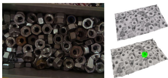
FIGURE 11. Reconstruction (top right) of a Bin of nuts (left image). The bottom-right picture shows detection of an item by a 3D Object Detection pipeline [48].
