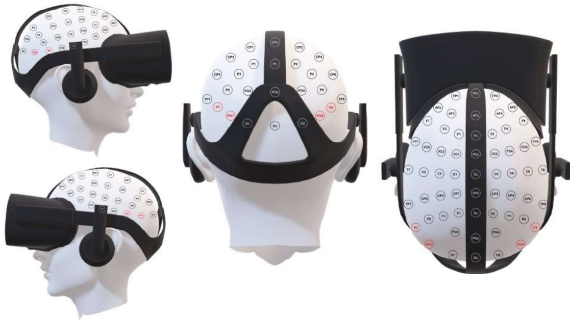
Figure 3. Illustration of the EEG/VR montage. As it can be seen in the illustration, the VR
