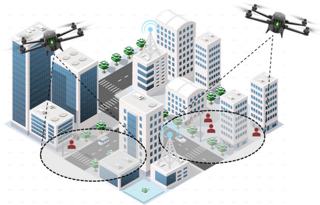
Figure 2. Example of an Aerial Base Station scenario for 5G services. The use of UABSs might be an efficient complement to traditional Terrestrial Base Stations (TBSs) or might even substitute TBSs in emergencies.
