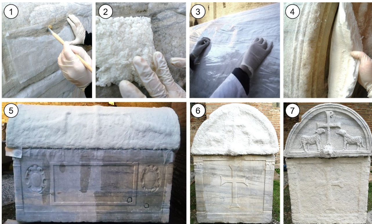
Figure S1. Consolidation of the sarcophagus by ammonium phosphate: (1) application of Japanese paper onto the marble surface by wetting with the DAP solution; (2) application of the poultice imbued with the DAP solution; (3) wrapping with a polyethylene film to prevent evaporation; (4) removal of the poultice after 24 hours; (5) view of the cover after application of the poultice; (6) view of the cover after wrapping with the polyethylene film; (7) application of the poultice onto the lower part of the sarcophagus.
