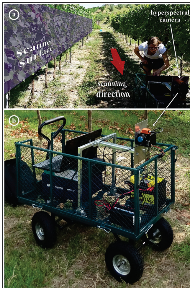
Fig. 2 (a) In-field hyperspectral imaging to measure soluble solids content of wine grape berries during ripening. In the picture a vineyard row, highlighted by the purple surface, was scanned with a Vis/NIR hyperspectral camera: the red arrow indicates the direction of scanning. The vineyard is located near Cesena, Italy. (b) Cart adopted for hyperspectral image acquisition.
